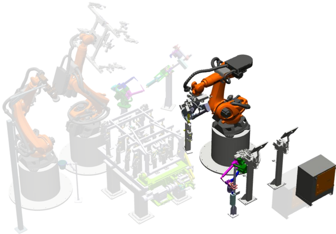
Figure 24 Robot with mounted and stationary welding tongs incl. Control cabinet
