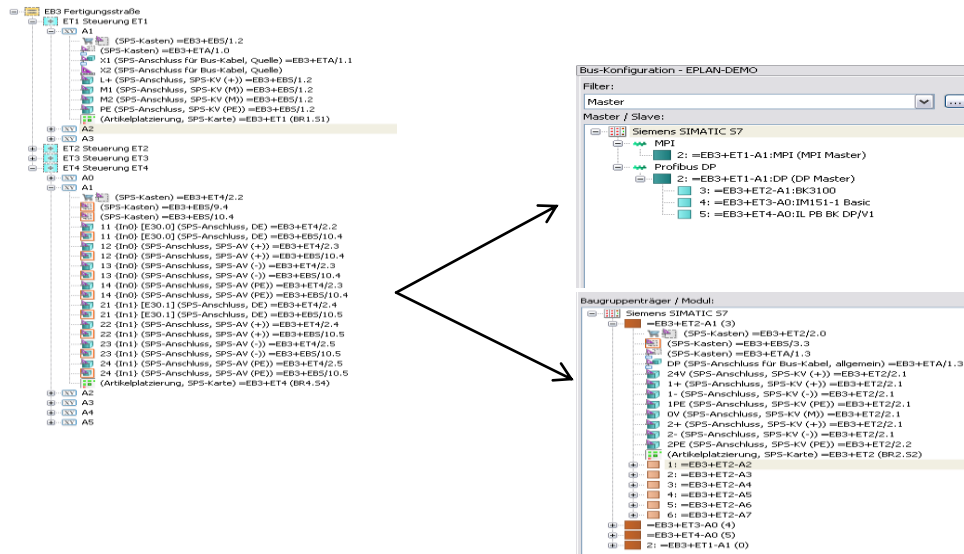
Figure 4 – Example for stations and bus data configuration
