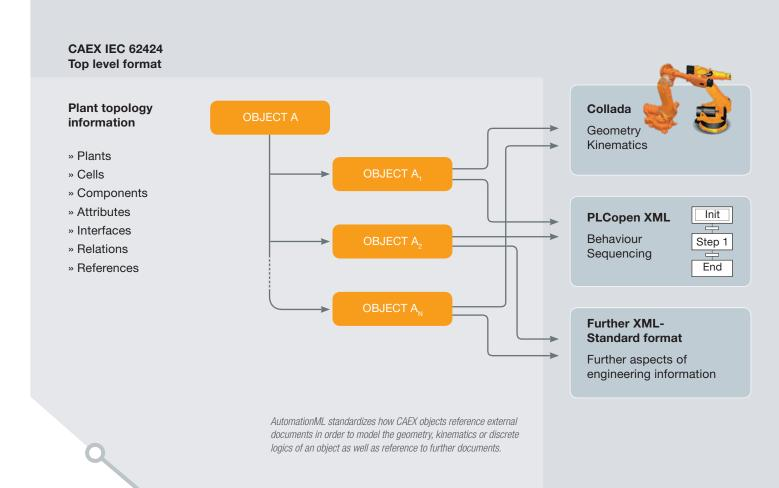
AutomationML combines existing established XML data formats which have been proven in use for their specific domain.
