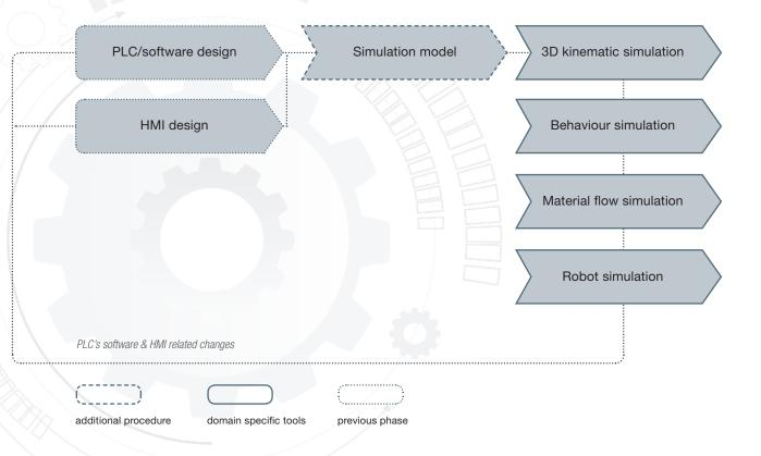
Based on practical experience, the 3D simulation model created and used by virtual engineering is taken as a base in order to use it for VC. In the market, several tools provide required functionalities to prepare the 3D simulation model and to conduct VC, e.g. DELMIA, Process Simulate, NX-MCD, RF::SGEdit, RF::YAMS etc.
