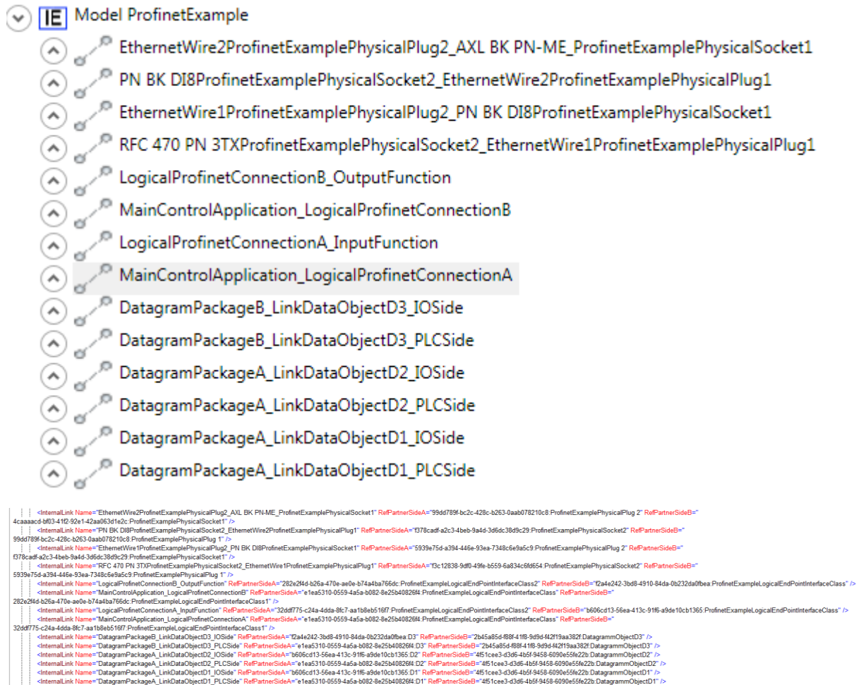
Figure 75 - Internal links related to the instance hierarchy for PROFINET demonstrator example
