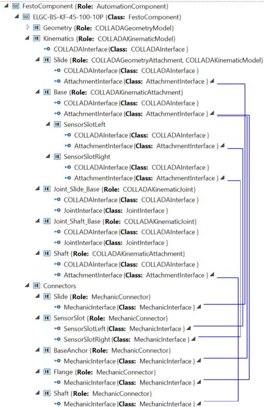
Figure 157: SystemUnitClass describing the drive with its geometry and kinematic model
