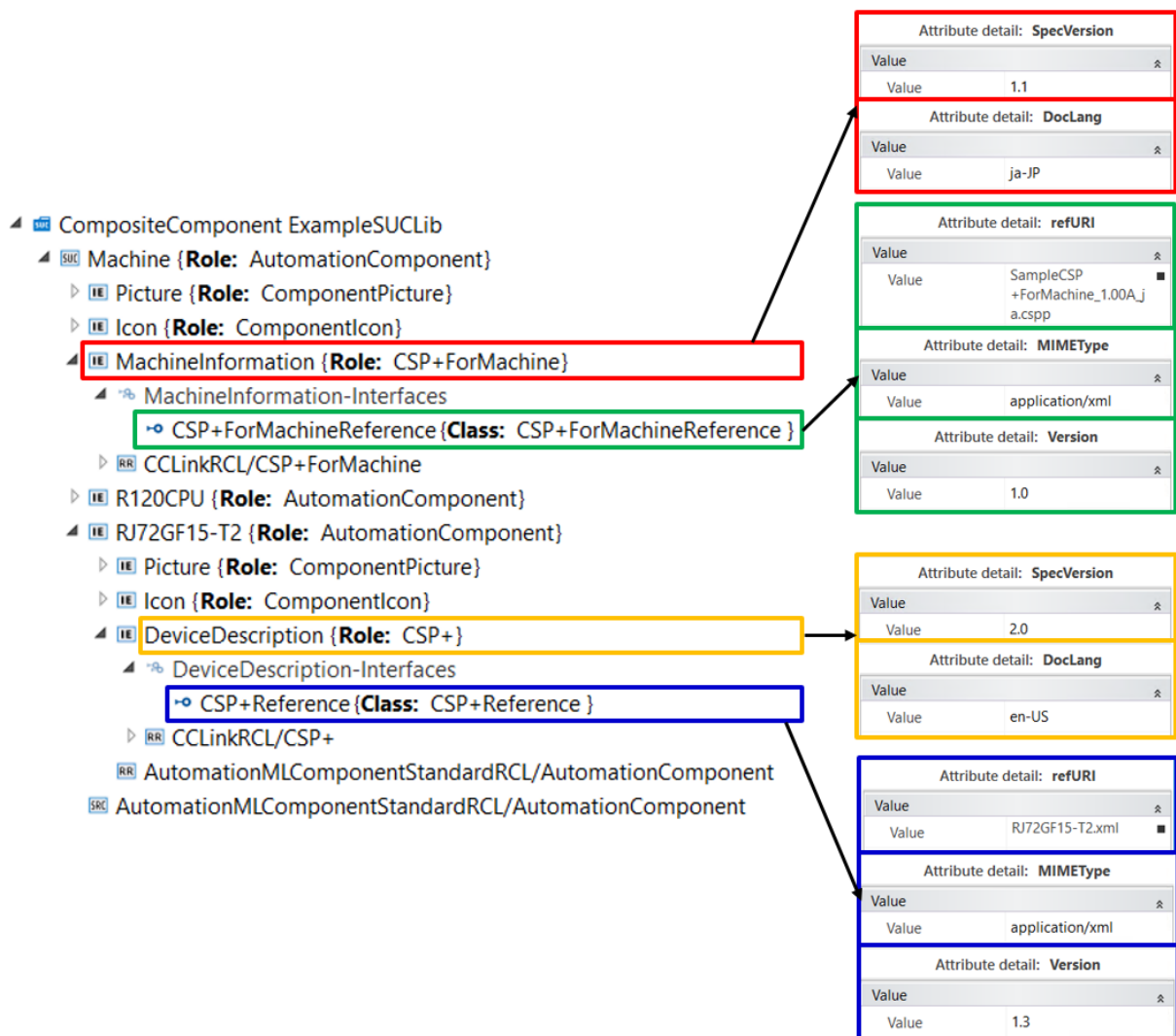
Figure 7 – Example “AutomationML Model including references to CSP+ and CSP+ for Machine” within the AutomationML Editor
